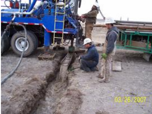
Photo: Powertech workers collect a Rotary Drill Sample at the Dewey Burdock site in March 2007. (Photo courtesy of www.powertechuranium.com ) -----
